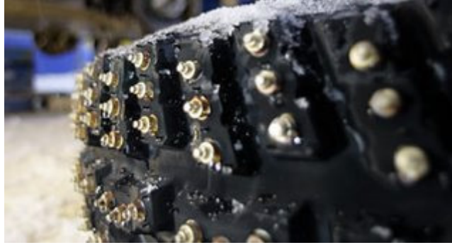
Fig. 2.2.1.1.2.d – Exemplary applications of standard 1.1.2 to snow tyres (internal additives = spikes)
