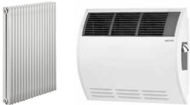
Fig. 2.2.2.1.2.e – on the left a radiator; on the right a convector: within there is a radiator and a fan to move quickly warmed air.
