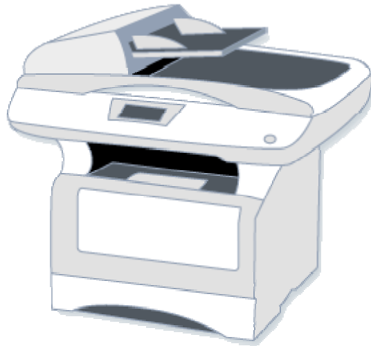
Fig. 2.2.3.1.1.c – a multifunctional printer: it is a poli-system composed by a printer, a scanner and a fax.
