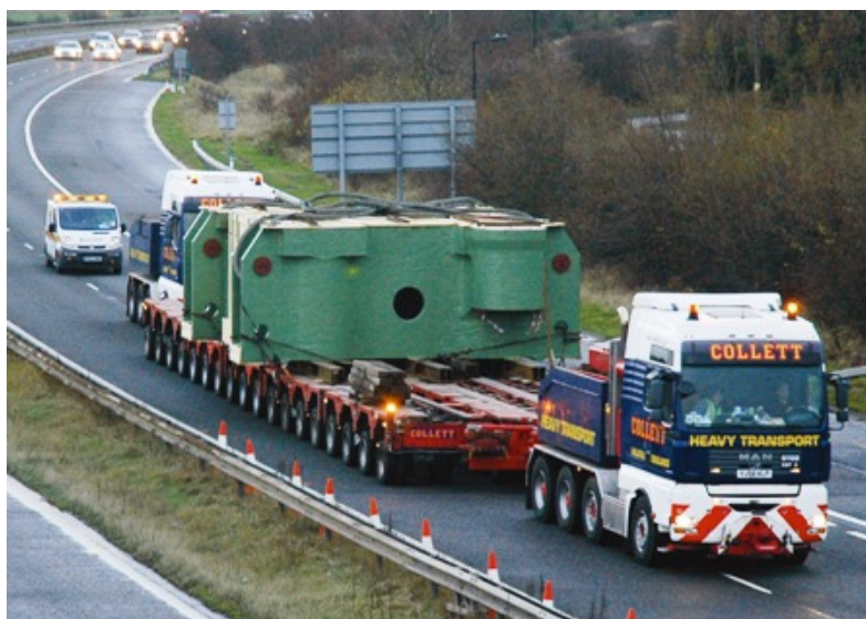
Fig. 2.2.3.1.1.b – in the image a trailer with axles evolved toward a poli-system
