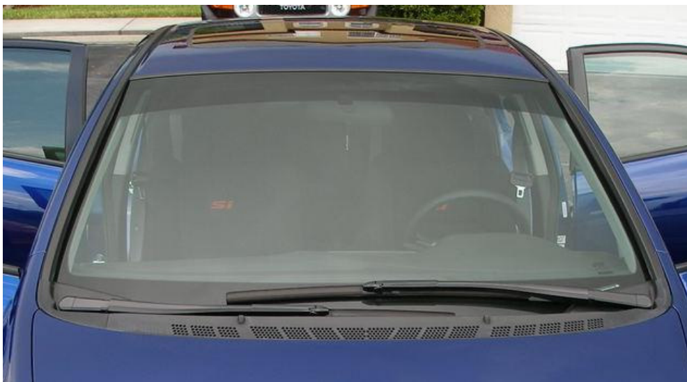
Fig. 2.2.1.1.8.1.c – on the top of the windshield the sun strip is visible; it lets see through but the sun is no more inconvenient because it is darker than transparent windshield glass.
