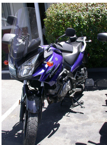
Fig. 2.2.3.1.2 – in the picture the two stands: the first (the center stand) sustain the motorcycle, while the second could avoid the first closure.
