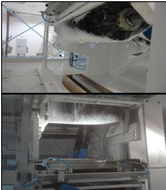
Fig. 4. Electrospinning: Application of a wooden reservoir (above), and a glass reservoir (below)
