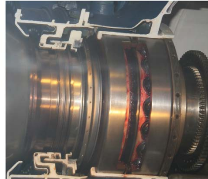
Fig. 2. (a) Roller bearing assembly. (b) Ball bearing No. 4. Picture courtesy of Museum Science & Industry Chicago.
